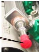
10. Fit 2 off PR1770 EP-14 yellow caps to the sump oil pipes.
