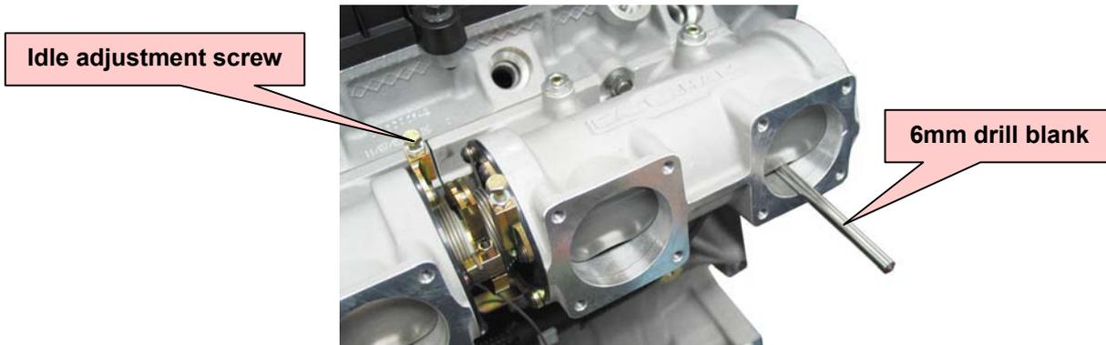
8. Using the 6mm drill blank now set the idle gap on cylinders 1 and 2 using the balancing adjustment screw.
