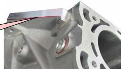
**Inspect head feed oil drilling for burrs**
