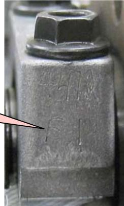
6. Torque each cap in the order shown below, initially to 7Nm then a final torque of 16Nm.
