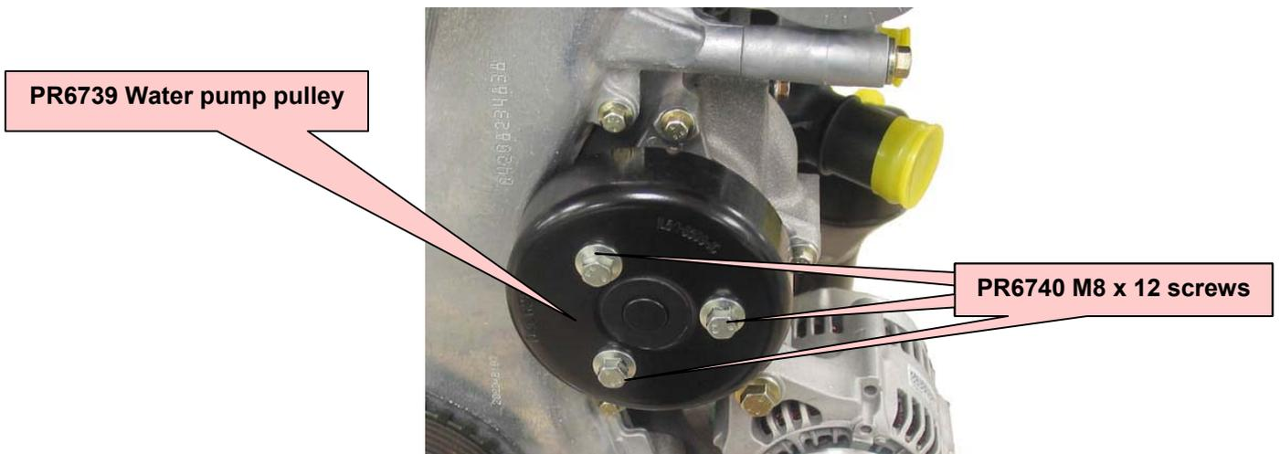
**Note:** - Ensure the drive belt running surface is kept clean.
