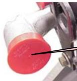
9. Fit PR1752 EC-M8 red cap to the fuel rail.
