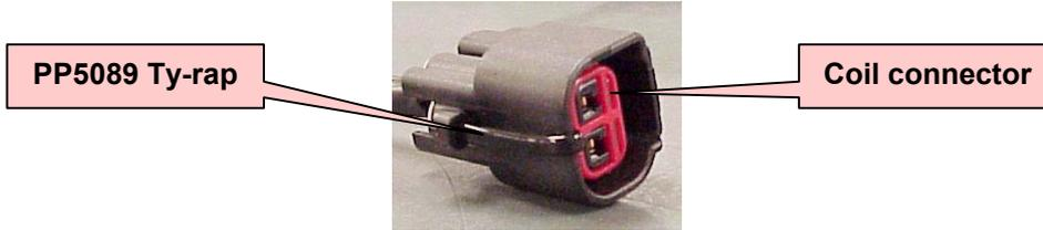
2. Fit YD8097 ignition coil loom to the engine and secure to 1 off PR6938 post using 2 off PP5089 Ty-raps.
